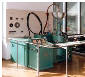
1958: The first electron beam welding machine (55kV) manufactured by Karl-Heinz Steigerwald.
